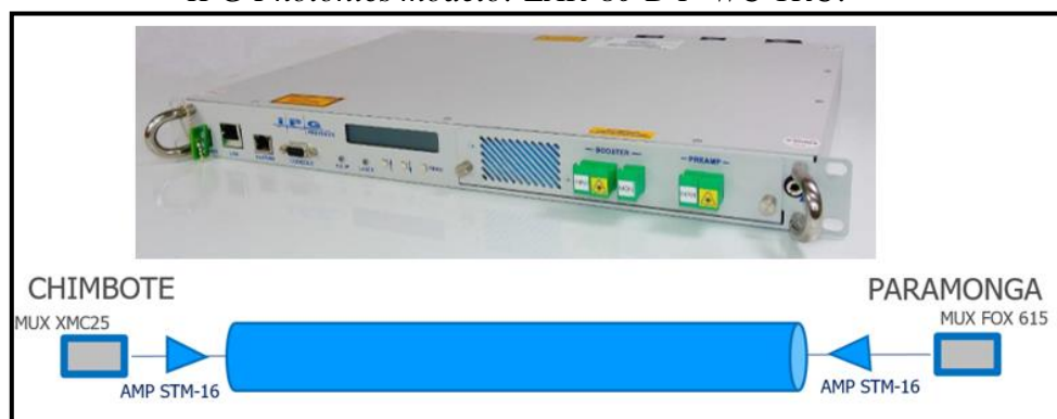
Figura N°15: IPG Photonics modelo: EAR-80-B-P-WC-1RU.
