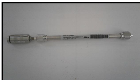
Figura 12: Columna LiChrospher100 Hibar RP-18 150 x 4.6mm, 5um Merck Millipore
