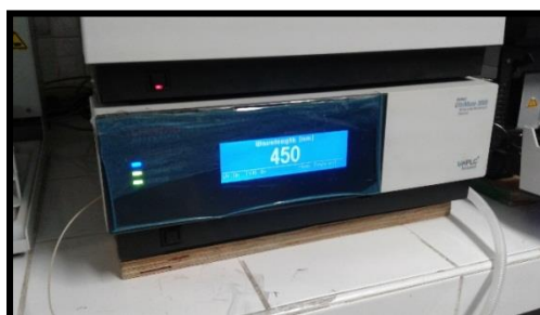
Figura 11: Detector UV-VIS UltiMate 3000 Thermo Scientific
