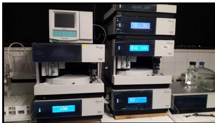
Figura 10: UHPLC UltiMate 3000 Rapid Separation Binary System Thermo Scientific
